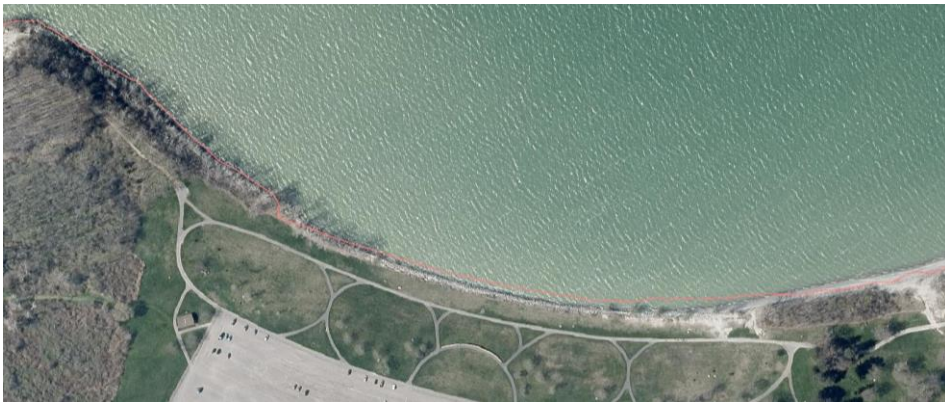
Photo 3: Hamlin Beach State Park from Devil's Nose East. Natural steep shoreline edge transitions to a rip rap reinforced shoreline for about 1000' between parking/lawn area and water.
