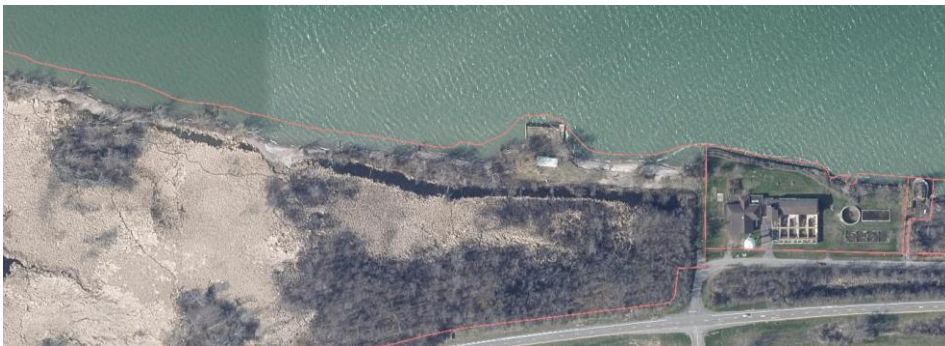
Photo 8: East edge of Hamlin Beach State Park is not reinforced. The Monroe County Water Authority Property at the east edge of the photo has shoreline walls and gabion shore protection that are in a state of disrepair.
